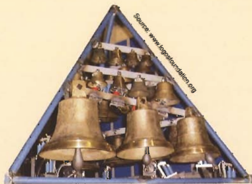
"Belly," Godfried-Willem Raes's programmable automated brass carillon with thirty-four bells
